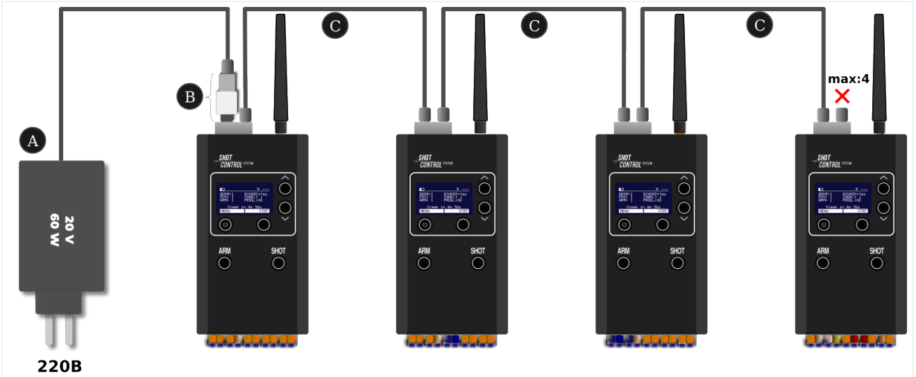
Figure 19: Charging 4 SBOX-30 devices
